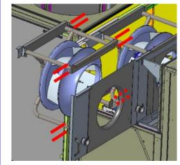
STEP 3: Remove screws 1-8 securing sides of fan to orifice and screws 9&10 securing rear bracket. Then carefully lift and pull the fan assembly from the orifice.
