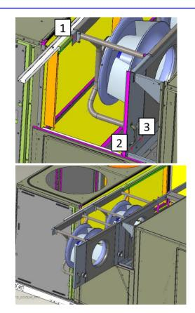
STEP 2: Remove 3 screws securing fan assembly. Then slide out ID fan assembly, to gain access to screws securing fan to orifice. (see next slide) Caution do not slide assembly beyond tipping point.
