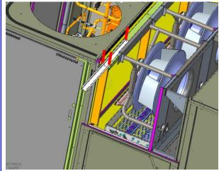
STEP 1: Remove 3 screws, relocate fan slide out bracket and resecure with 3 screws
