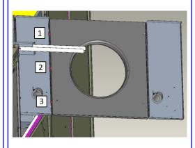
STEP 4: Remove 3 screws securing front block-off and orifice to access removal of the second fan assembly
