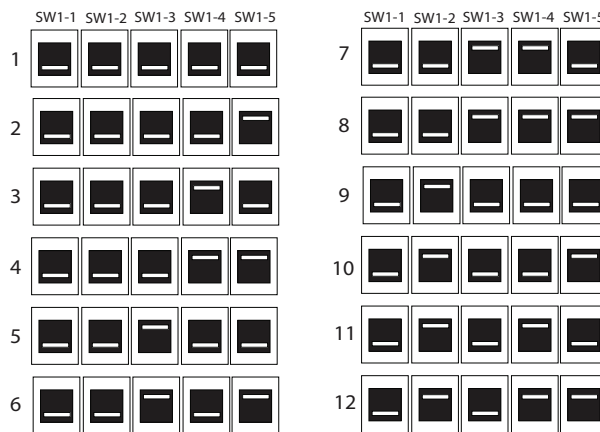
Figure 10. Comm 3/4 communications module address setting for VariTrac I comfort manager and VariTrac II central control panel — ALL address numbers and ReliaTel communications interface board DIP switch settings
