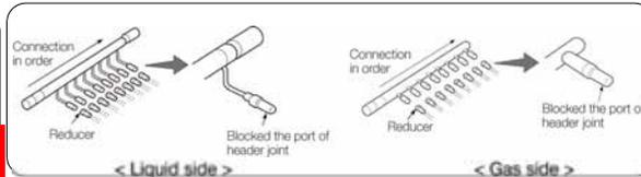
Install the header joint horizontally.
