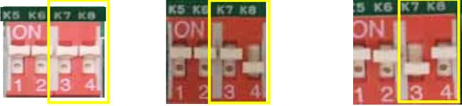
On/On : Main Unit    On/Off : Sub Unit 1    Off/On : Sub Unit 2
