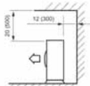
When front and back of unit are blocked by walls
