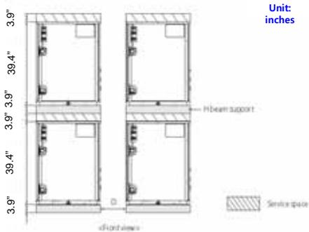
If the WCU needs to be installed close to the walls, prevent vibration from being transferred to the walls with cushioning materials, etc.
