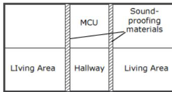
Reduced risk of noise transfer by utilizing interior walls to isolate MCU from occupied spaces.
