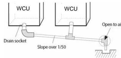
1. Attach the drain pipe to the drain socket (PT1/2) located on the bottom of the product.
