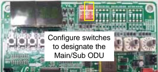
Configure switches to designate the Main/Sub ODU
