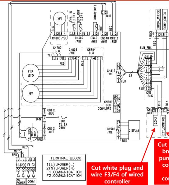
Cut red, 4 wire plug to interlock "something" to unit operation (erv, etc.) and/or to utilize the "error check" function.
