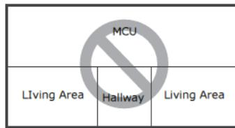
Increased risk of noise transfer from MCU to occupied spaces because of the free flow of sound between occupied spaces.
