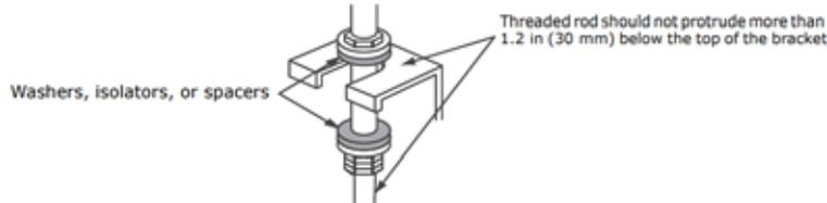
8. Maintain proper spacing between the unit and the ceiling; refer to the following figure.
