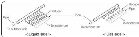
Braze ends of the pipes with caps which are not occupied
