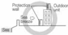
▶ Protection wall should be constructed with a solid material such as concrete to block the sea breeze and the height and the width of the wall should be 1.5 times larger than the size of the outdoor unit. Also, secure over 27" between the protection wall and the outdoor unit for exhausted air to ventilate.
