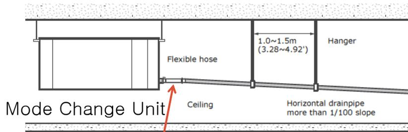
Accessory Drain Hose Stub gravity drain only, can drain to central point for pumping.
