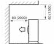
When top of unit is blocked and the air outlet is opposite the wall
