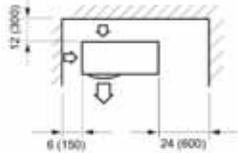
Top of unit is blocked and the air outlet is toward a wall
