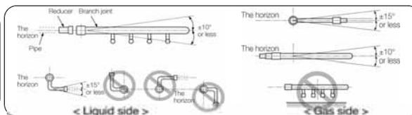
Incorrect installation of Y-joint & Header Joint cause poor oil and refrigerant distribution between IDU's. It may decrease the system's performance or cause compressor failure.
