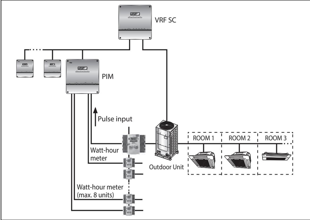
A maximum of 8 PIMs can be connected to a VRF system controller.
