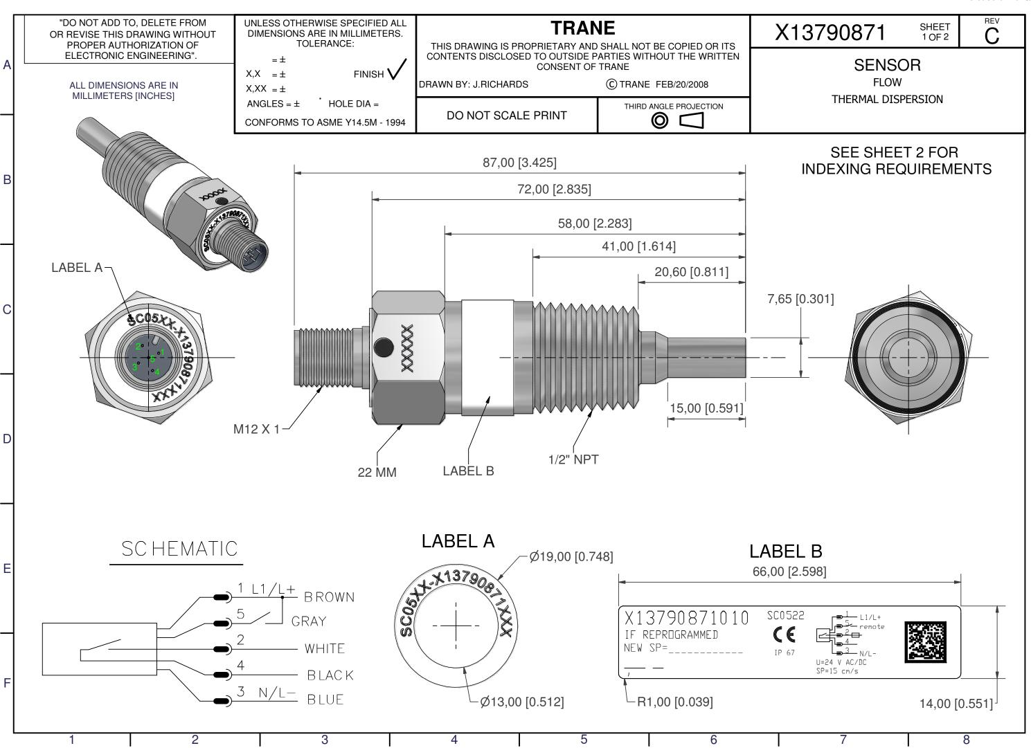
SHEET 2 OF 2 "DO NOT ADD TO, DELETE FROM X13790871 C OR REVISE THIS DRAWING WITHOUT PROPER AUTHORIZATION OF ELECTRONIC ENGINEERING". **INDEXING REQUIREMENT** ALL DIMENSIONS ARE IN MILLIMETERS [INCHES] NOTE: 1. INDEXING REQUIREMENT REFERS TO INSTALLING THE FLOW SWITCH INTO THE PIPE SUCH THAT THE DIMPLE ON THE HEX FLAT IS FACING DIRECTLY INTO THE FLOW WITH A TOLERANCE OF +/- 90°
