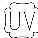
FIG. UG-129.1 OFFICIAL SYMBOL FOR STAMP TO DENOTE THE AMERICAN SOCIETY OF MECHANICAL ENGINEERS’ STANDARD FOR PRESSURE RELIEF VALVES
