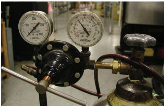
Figure 3. Two-stage nitrogen regulator
