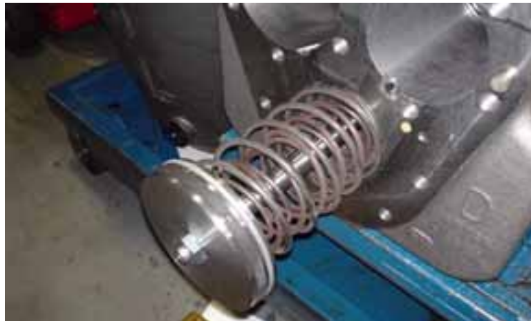
Figure 14. Installing the Piston
