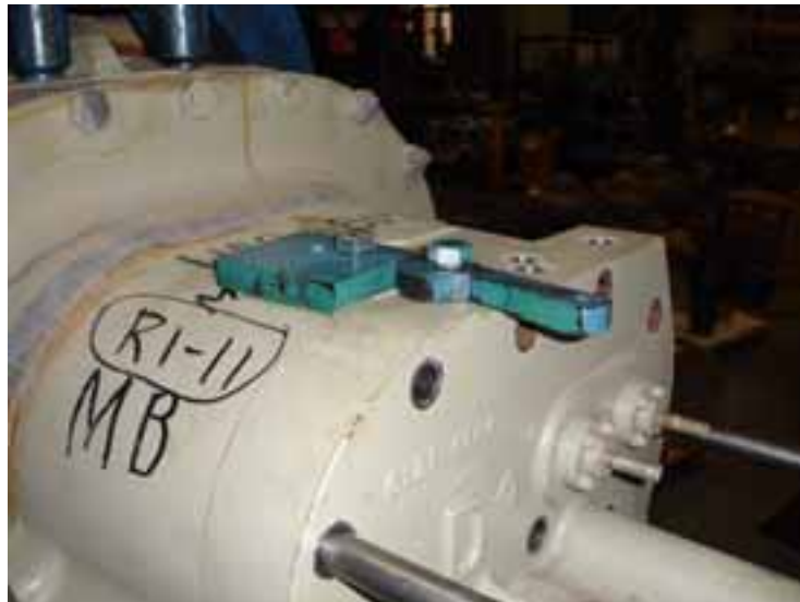
Figure 10. Install Metal Plate and Cam - handle
