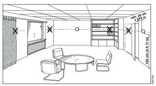
• The room thermostat must be mounted in a clean, dry indoor place and must not be exposed to drip or splash water
