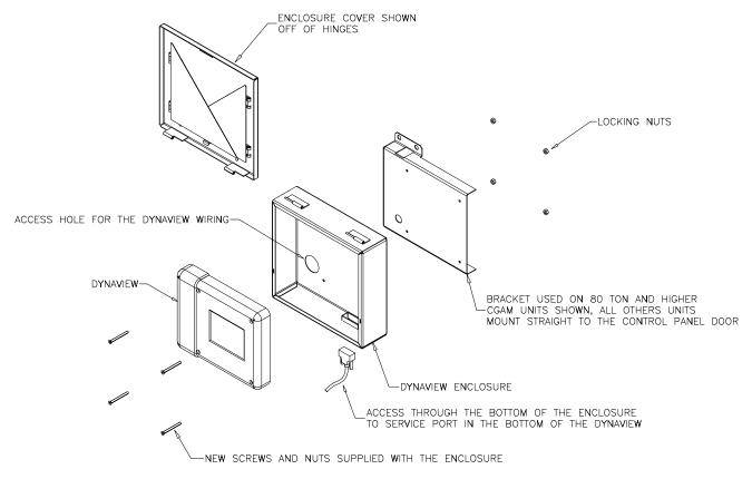
6. Slide the DynaView enclosure cover back on its hinges and prop it open by sliding the side shields into the slots.
