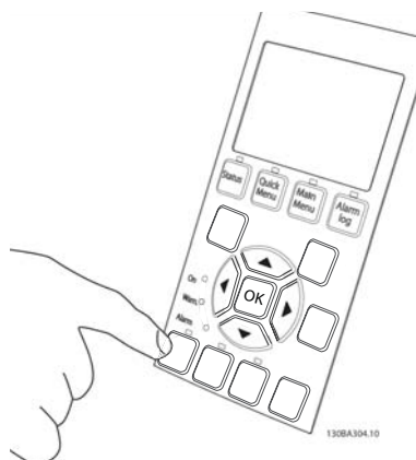
Figure 4.47: Step 5: By pressing the [Hand on] button, the LED above the button should be lit and the motor may rotate.
