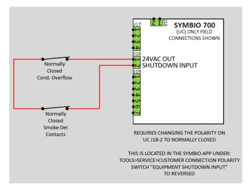
Wiring above reflects normally closed safeties. Typically, condensate overflow switches (or pan switches) are normally closed devices. If using normally open devices, they can be wired in parallel, and the Customer Connection Polarity does not need to be changed.
