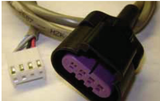
Figure 11. Procure locally - White four place screw terminal connector (used on CTV Industrial option INDP)
