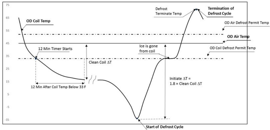
During the defrost cycle, the Switchover Valve is turned ON, the Condenser Fan is turned OFF, and auxiliary heat is turned ON regardless of their prior operating status while maintaining compressor operation. The defrost cycle is terminated based on the defrost termination temperature calculation using the outdoor temperature (ODT) +47°F. The defrost termination temperature (DTT) will be limited between 57° F and 72° F.
