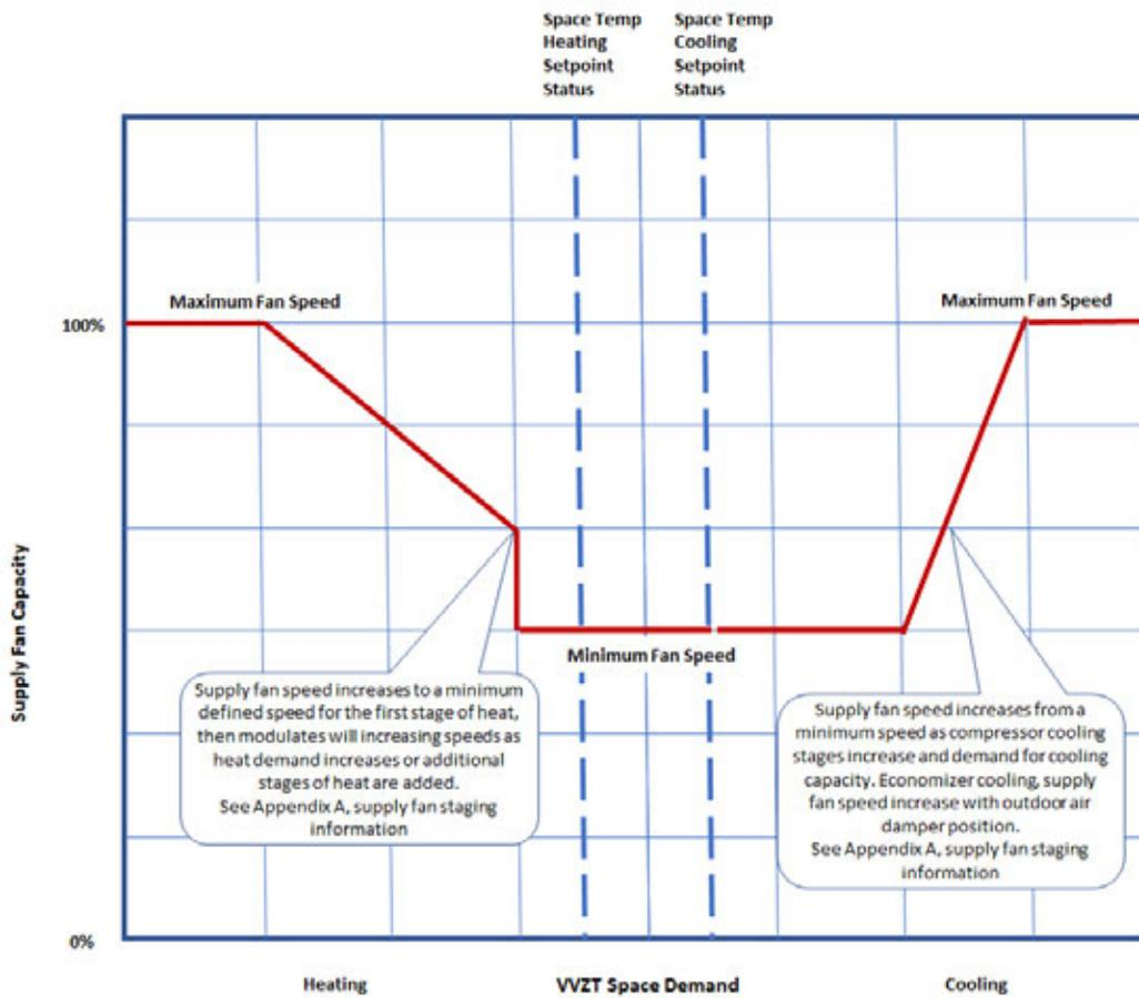
Figure 11. Supply fan operation - heat pump heating and cooling
