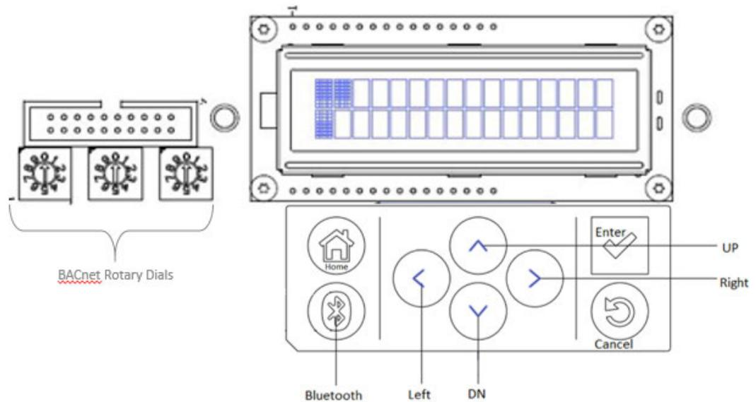
The interface provides an intuitive menu structure: alarms, status, service, settings, and utilities. Configuration of the unit is accomplished under the utilities menu item. A complete list of functions is outlined in *User Guide, Symbio™ 700 (BAS-SVU054\*-EN)*.
