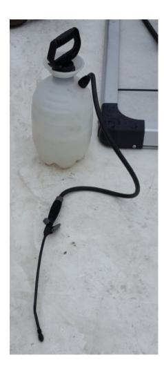
Common garden sprayer was used to apply cleaning mixture.
