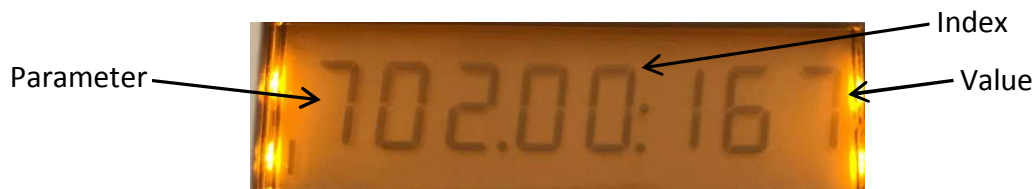
Figure 7-1: LME7 Fault History Example with Indexes
