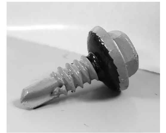
ITEM# 3 SCREW; .250-14 X .75 LEACHED SELF DRILLER WITH PLASTISOL
