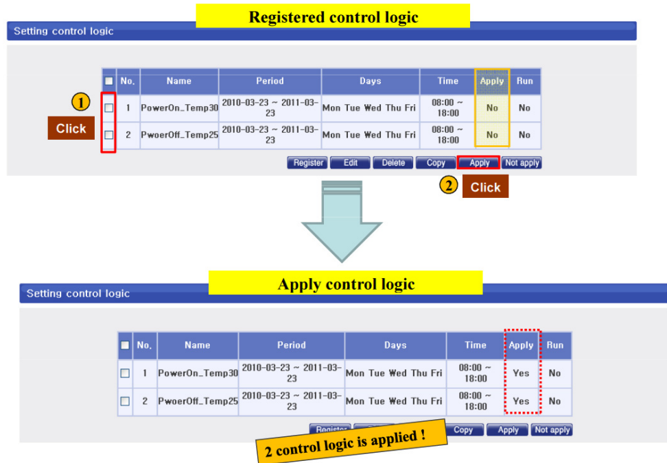
Figure 22. Custom control logic applied to indoor units
