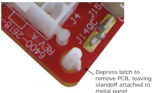
Figure 63. Remove PCB
