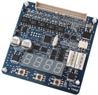
Figure 18. VelociTach motor control board
