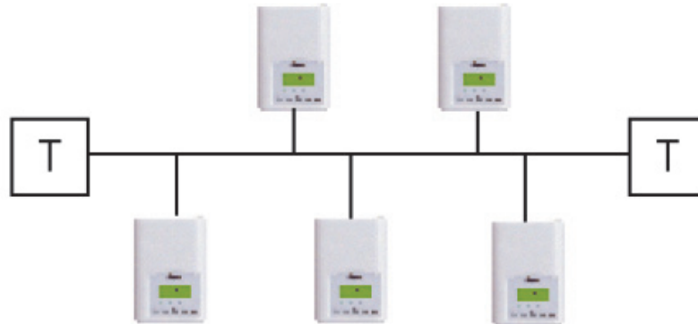
Figure 6. Doubly terminated bus topology
