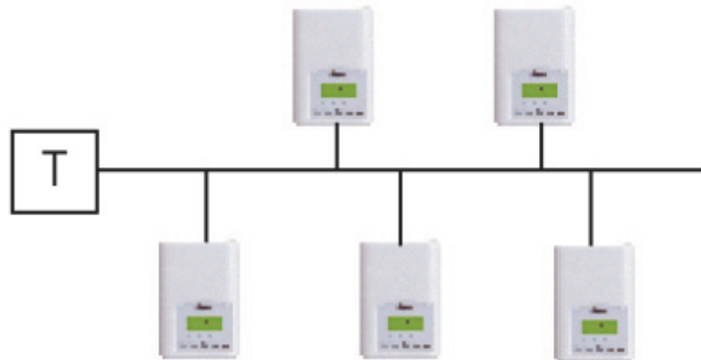
Figure 5. Singly terminated bus topology
